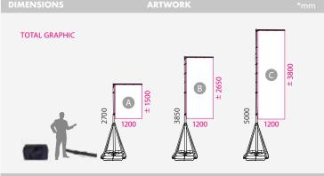
The Bejar is a telescopic flagpole adjustable to 3 heights: 2700, 3850 or 5000mm with a refillable 76l plastic base. Its feet structure is foldable and its base is 4-pieces removable for an improved storaging. Bejar flagpole is made of aluminium and plastic parts. 2 carry nylon bags are included for a better transportation. Ideal for being used at outdoor events, tradeshows, exposition entrances or just for displaying to largue distances.
