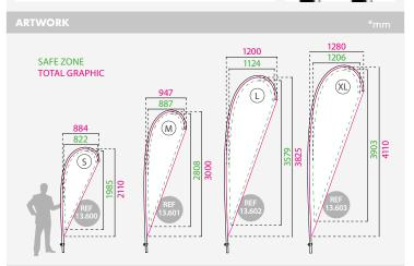
The Spoon model is a flagpole made of fiberglass, aluminium and plastic. The pole is collapsible for an easy portability. Also, a carry nylon bag is included. Multiple accessories are available later at this chapter. Textile manufacturing available (not included). You can choose A white or **B** black colour of pole sheath.
